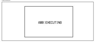
The black balance adjustment ends in a few seconds with the message "ABB:OK" and the adjustment setting is automatically stored in memory.
